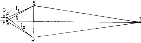
Fig. 27-9. The resolving power of an optical system.
